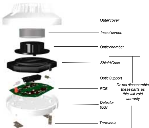
Figure 1:- 'Exploded' View of ST-P-AS sensor Assembly
